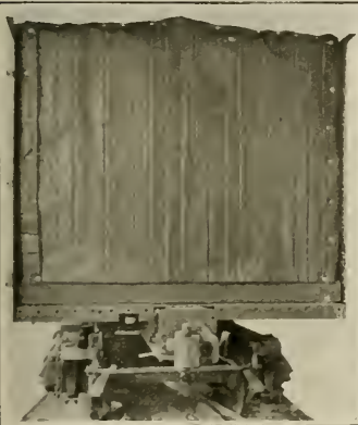
END VIEW P. R. R. REFRIGERATOR CAR—SIDE SHEATHING PLACED.
